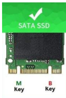
Figure 27 Example M.2 SATA SSD with B- and M-key coding
